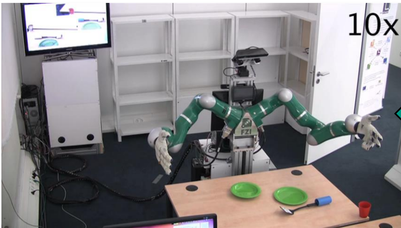
Execution using 2D-vision to localize objects
